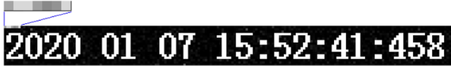
Figure 20: Time values that SharpCap records in the frame image. The values are superimposed on the image. The seven pixels at the top left corner contain the time since 0:00:00 A.D. in units of 10^{-7} as pixel data.
