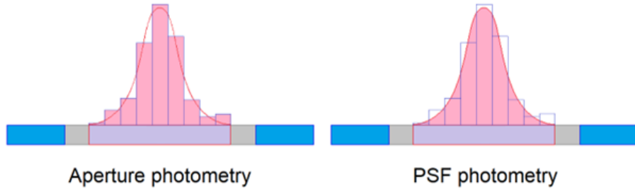
Figure 38: Aperture photometry and PSF photometry. Aperture photometry calculates the light intensity by summing the pixel values within a measurement region, while PSF photometry calculates the light intensity as the integral of a rotating Gaussian curve that approximates the peak of the pixel values. Aperture photometry is suitable when atmospheric turbulence causes large deformations in the star image (pixel value distribution deviates from the ideal state). On the other hand, PSF photometry can reduce noise over time.
