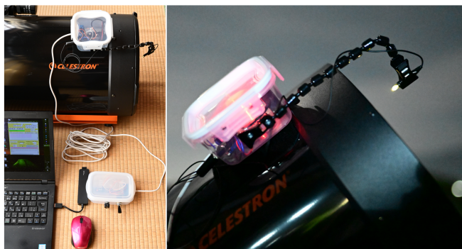
Figure 33: Example of a self-made receiver (left) and its installation at the front of the telescope tube (right)
