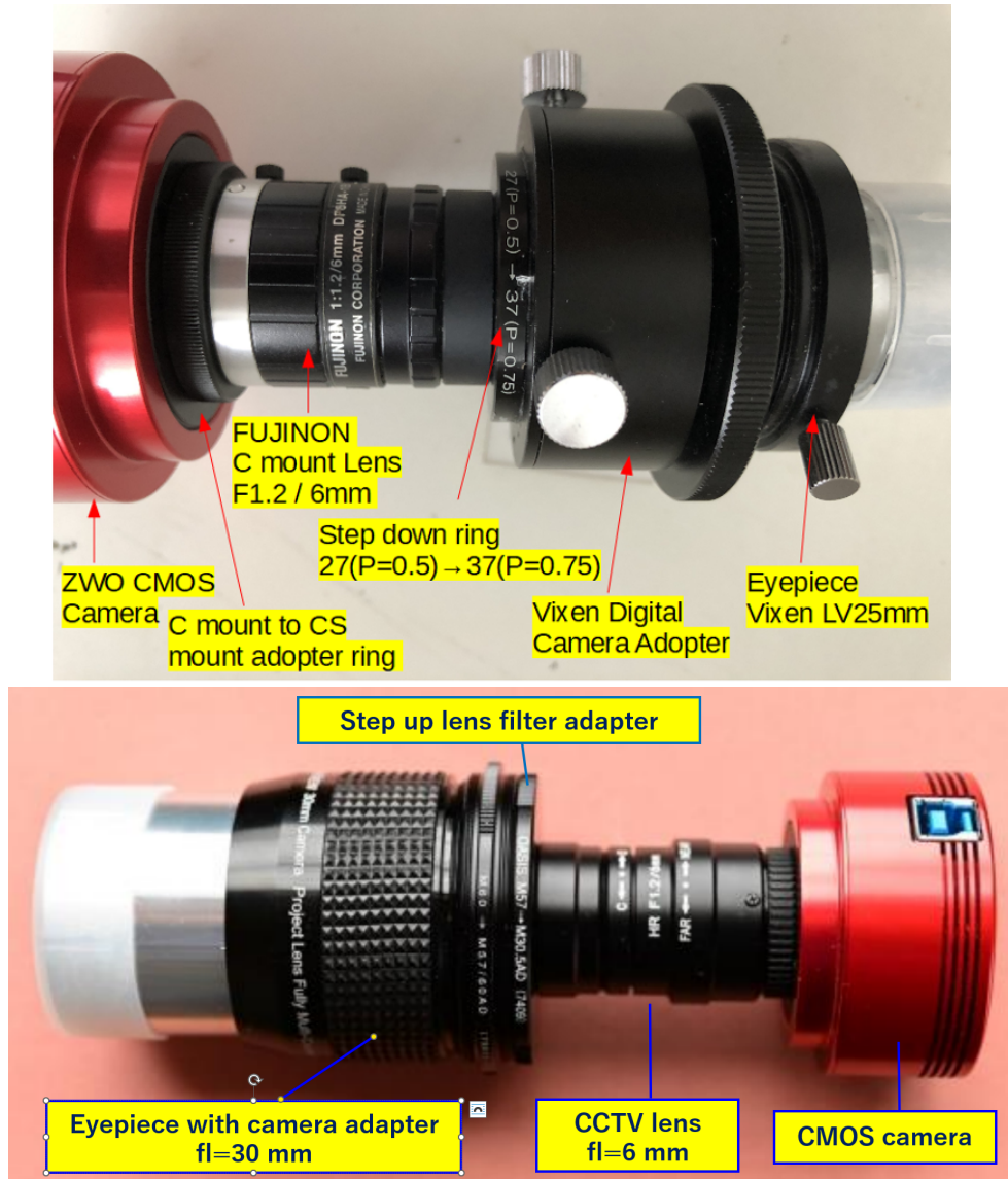
Figure 29: Example of a reduced optical system configuration using the collimation method
