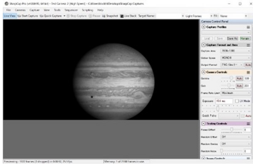
Figure 27: SharpCap4.0 Display of image captured by connecting test camera 2 (high speed)
