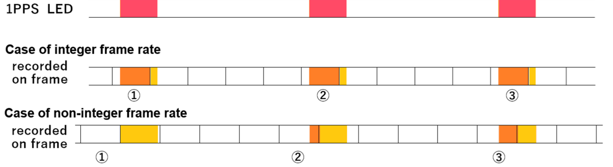
Figure 23: The frame rate and the recorded 1 PPS of LED light. The middle bar shows 5.0 fps (integer fps), and the bottom bar shows 4.45 fps (not an integer fps). The light intensity of the LED light recorded to a frame every turning ON the LED. When the frame rate is an integer, the light intensity remains constant. However, when the frame rate is not an integer, the brightness changes at a constant rate.
